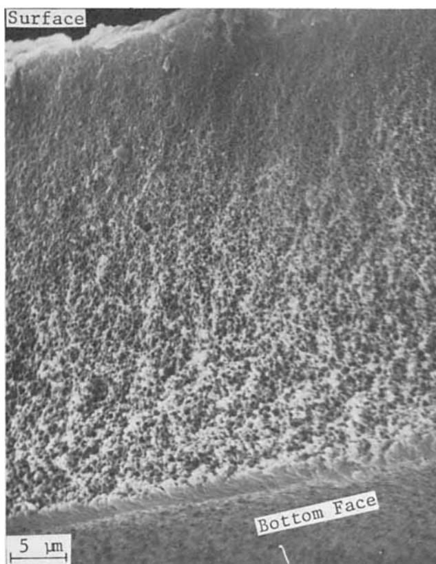
Fig. 6. Cross section of PVPy/CA (formula index 8a) alloy membrane.
