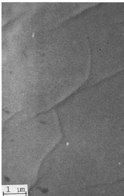
Fig. 8. Scanning electron micrograph of asymmetric PVPy/CA membrane (formula index 8a) showing surface of a membrane dried under ambient conditions. The membrane shrank less than 1% of its original size, displaying subtle wrinkles at the skin face. Although the overall flux rate of such a membrane decreases (~50%) the membrane retains its separation capability (~90% SR at 200 psi).
